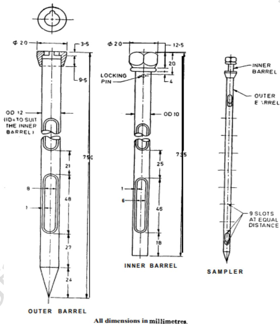
Fig. 1 Typical sampler for formulations in solid form
